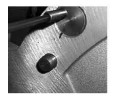
MARK THE PLATE FOR ANY ADDITIONAL TRIMMING OR CUTTING FOR CLEARANCE. IF THE PLATE WILL BE TRIMMED, BE CAREFUL NOT TO CUT TOO CLOSE TO ANY OF THE FASTENER HOLES AND REMOVE ANY BURRS LEFT FROM CUTTING.
